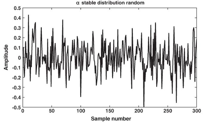
Fig. 2.  $S\alpha S$  pseudoreflectivity coefficient with  $\alpha = 1.8$ .
