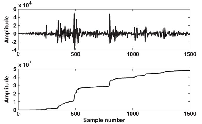
Fig. 15. Real seismic data and their running sample variance.
