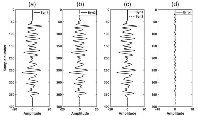
Fig. 13. Synthetic trace error analysis on the recovered Ricker wavelet. (a) Synthetic trace generated by the true Ricker wavelet. (b) Synthetic trace generated by the estimated Ricker wavelet. (c) Two synthetic traces. (d) Error of the two synthetic traces.
