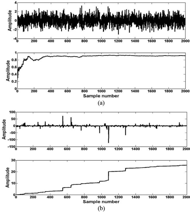
Fig. 14. Two sets of random  $\alpha$ -stable distributions and their running sample variances. (a)  $\alpha = 2.0$ . (b)  $\alpha = 1.4$ .
