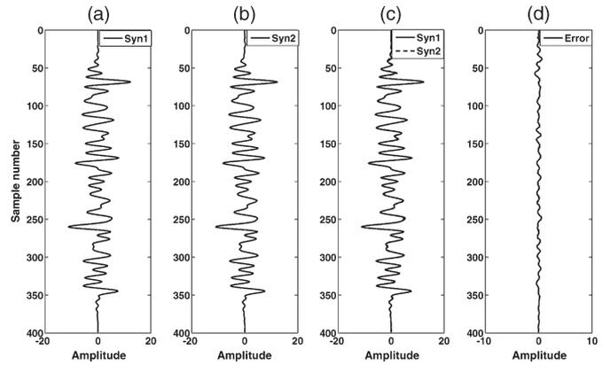
Fig. 12. Synthetic trace error analysis on the recovered bandpass wavelet. (a) Synthetic trace generated by the true bandpass wavelet. (b) Synthetic trace generated by the estimated bandpass wavelet. (c) Two synthetic traces. (d) Error of the two synthetic traces.
