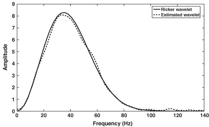
Fig. 11. Amplitude spectrums of the Ricker wavelet and its estimation wavelet.
