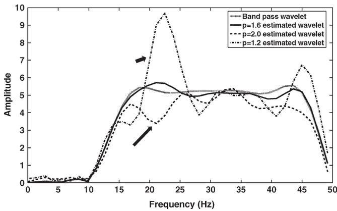
Fig. 5. Amplitude spectrums of bandpass wavelets with different moments.
