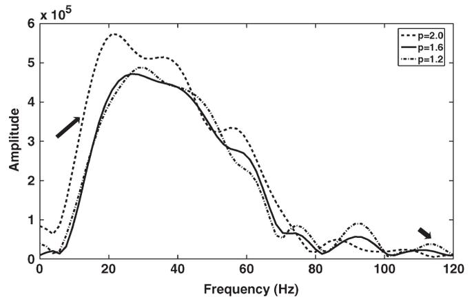
Fig. 19. Amplitude spectrums of the recovered wavelets from real data.
