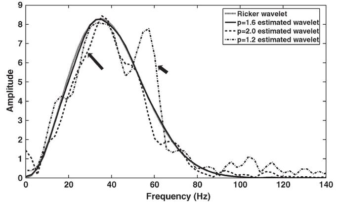
Fig. 7. Amplitude spectrums of Ricker wavelets with different moments.
