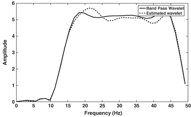
Fig. 10. Amplitude spectrums of the bandpass wavelet and its estimation wavelet.
