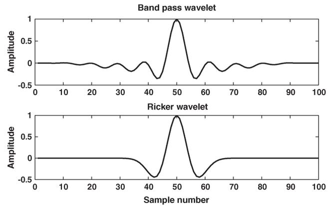
Fig. 3. Two types of wavelets. (a) Bandpass wavelet. (b) Ricker wavelet.
