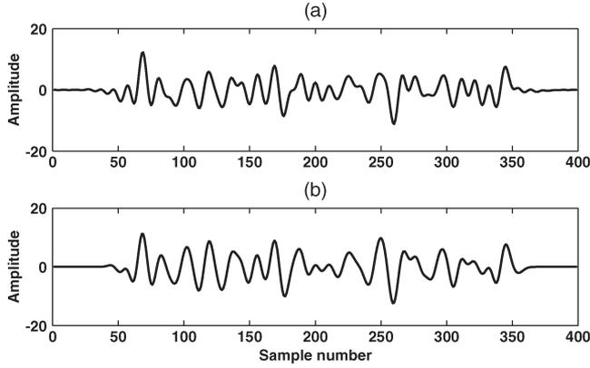
Fig. 1. Synthetic traces for wavelet estimation. (a) Generated by convolving a normalized  $S\alpha S$  pseudoreflectivity coefficient with a bandpass wavelet. (b) Generated by convolving a normalized  $S\alpha S$  pseudoreflectivity coefficient with a Ricker wavelet.
