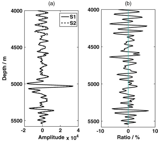
Fig. 20. Synthetic trace error analysis.
