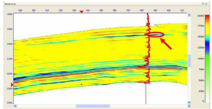
Fig. 23. Acoustic impedance inversion result.
